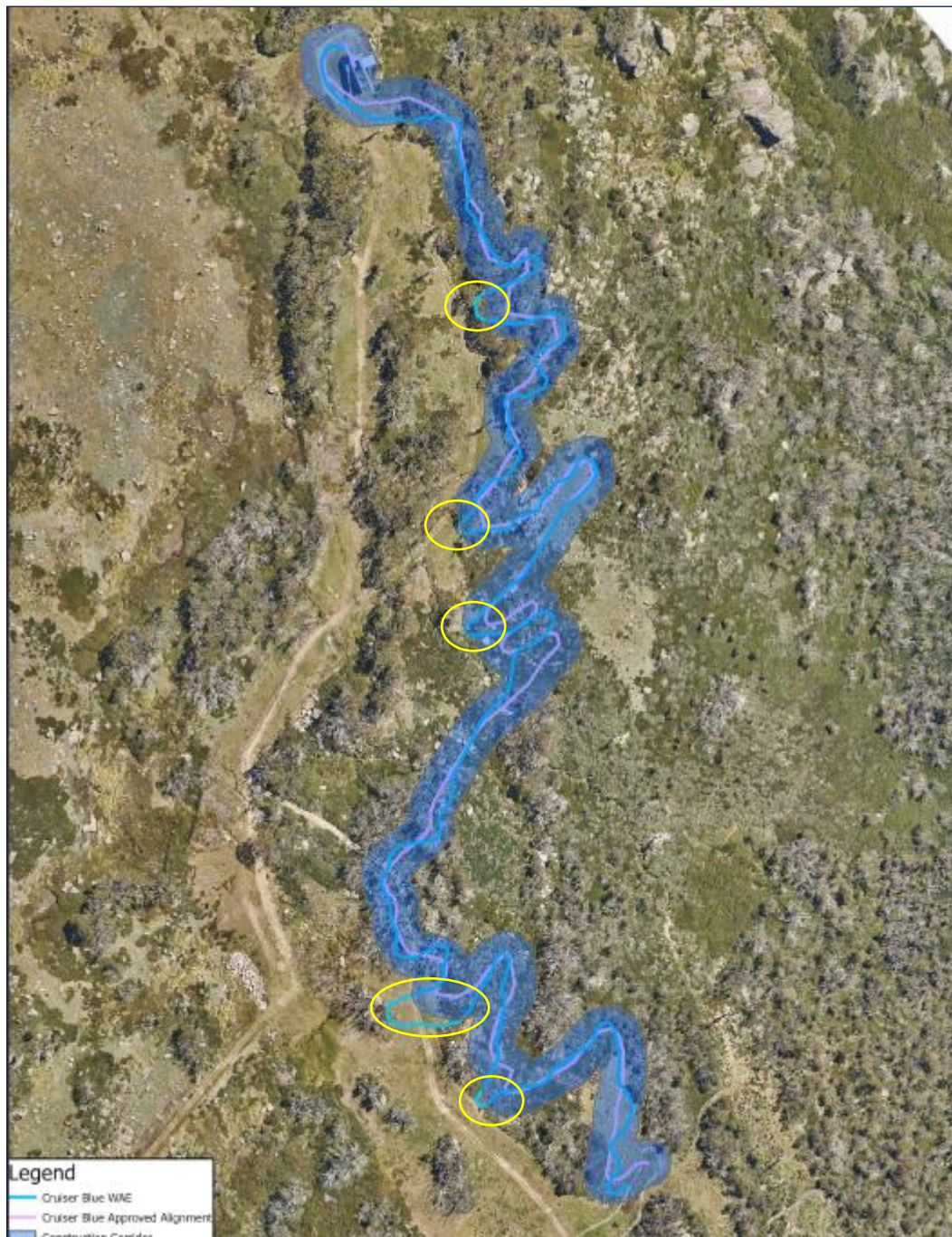
Figure 2: | Works as executed plan with construction corridor overlay indicating the five (5) areas constructed outside of the approved construction corridor (Source: Applicant's documentation)
